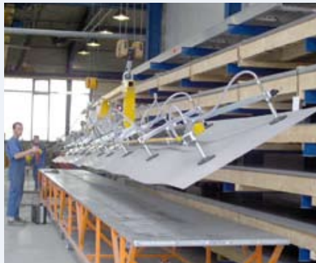
VacuBoy-90 handling thin steel plates
