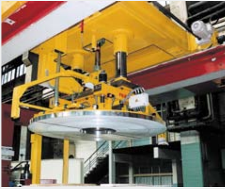
VacuCoil in automatic operation
