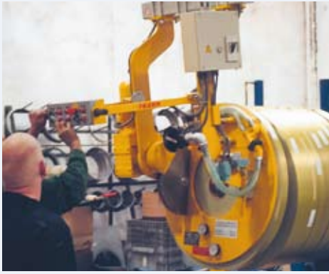
VacuCoil during removal process from a mandril
