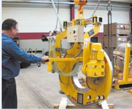
VacuCoil with flattened suction plate for the upright engagement of coils with various diameters
